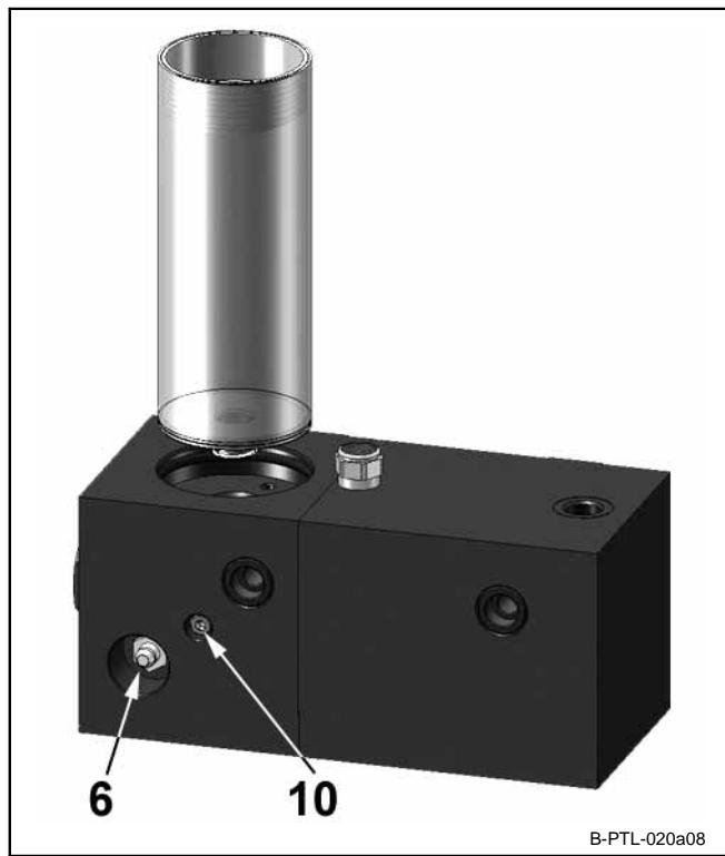
Fig. 8 Insert cartridge into lubrication pump PTL 201
