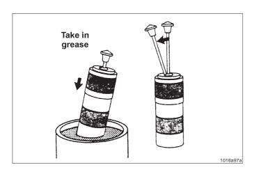
Immerse open part of pump reservoir into grease. Pull piston guide rod vigorously upwards and lock it into groove. Avoid air inclusions.
