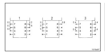
When outlet 7 and/or 8 closed, the output from either or both of these outlets, plus that of the immediately adjacent closed outlet 6 (see ex. 4) is redirected internally to the pump reservoir.
