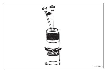
Screw reservoir ono pump. Release guide rode (central position).
