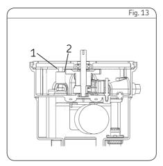
Switching parts of the low-level control for oil (when the reservoir is empty).
