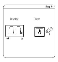
Press button to change value. Reading x 100 = Transducer setting in psi  $9 \times 100 = 900$  psi.
