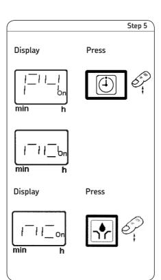
P4: Programming of the output signal for both alarm relays. The default setting on the printed circuit board for the alarm contacts is switching to battery minus.
