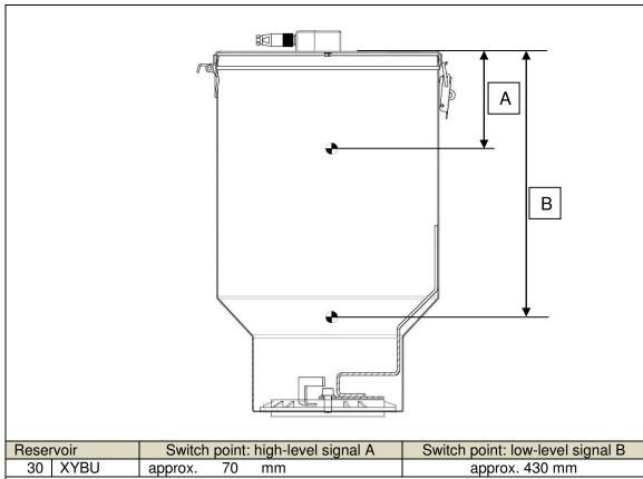
The minimum distance between the lubricant and the ultrasonic sensor totals 60 mm. If this
