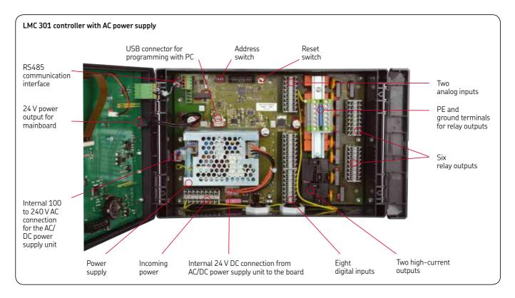
The LMC 301 utilizes pressure switches and pressure transducers, and a grease monitor sensor can be placed before the lubrication point to verify that the system is working correctly. This is ideal for use on critical bearings where it is essential to know that they have been lubricated properly.
