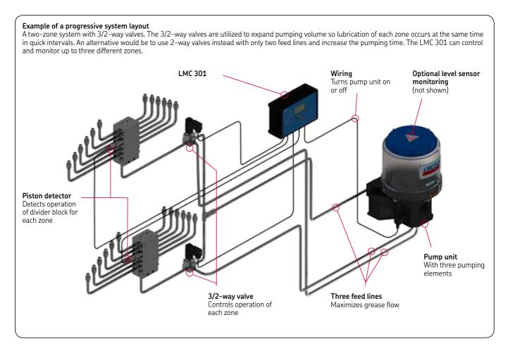
In progressive automatic lubrication systems, a piston pump supplies a defined amount of lubricant through the main line to the metering device that serves each outlet. SKF ProFlex and Lincoln Quicklub systems are designed for specific applications and can be configured to meet the unique requirements of every lubrication point on the equipment.
