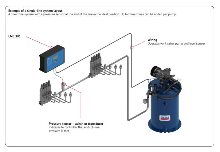
Regardless of the application, the principle of single-line lubrication remains the same: a central pump station automatically delivers lubricant through a single supply line to the lubricant metering device. Each metering device serves only one lubrication point and may be adjusted to deliver the precise amount of grease or oil required. Systems can service one machine, different zones on one machine or even several separate machines.
