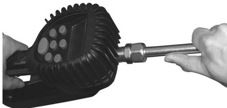
1. On the opposite end, apply sealant to the end of the nozzle. Recommended sealant is Loctite<sup>®</sup> 243.
