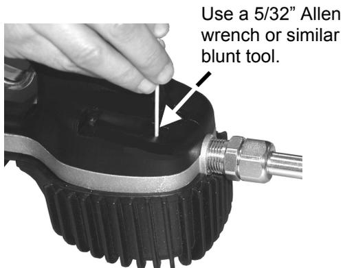
1. Press the **RESET** button to wake up the meter if the display is blank.
