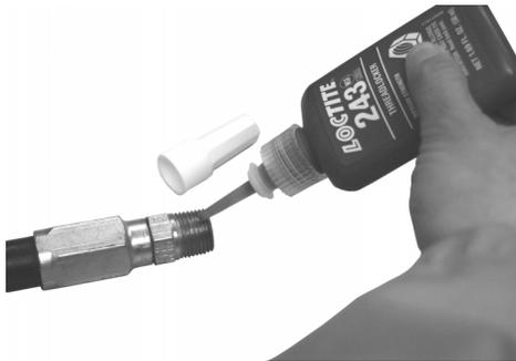
1. Attach swivel to meter. Apply thread sealant to the male end of the hose. Recommended sealant is Loctite<sup>®</sup> 243.
