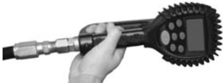
2. Insert the metal end of the hose into the swivel. Tighten completely with an open ended, adjustable, wrench.
