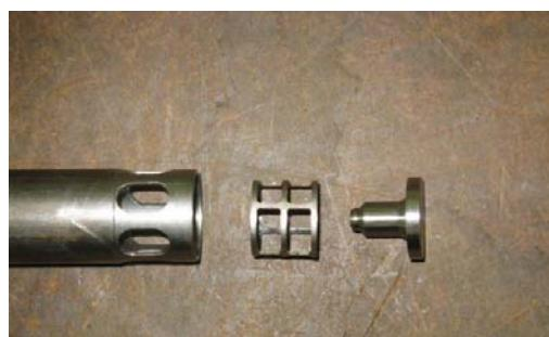
19. Exploded view of housing tube (Item 56a), spacer (Item 56) and Shovel Plug (Item 58).
