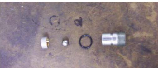
47. Remove ball cage (Item 24), check ball (Item 25) and O-ring seal (Item 26) from check seat housing (Item 27).
