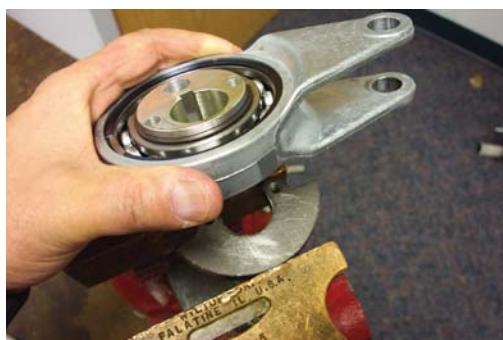
56. With both flat head screws removed, remove counterbalance weights (Item 2).
