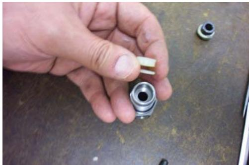
35. Remove cup seal (Item 15) and backup washer (Item 14a). (Reassembly recommendations: replace cup and seal and backup washer. See detail below for orientation.)
