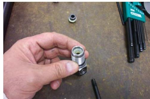
33. View of wrist pin anchor (Item 13a) showing upper cup seal (Item 15) and nylon back up washer (Item 14).
