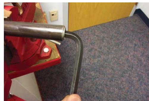
45. Loosen check seal housing (Item 27) with 3/8 Allen wrench. (Reassembly torque: 20-25 ft. lbs. (27.1 - 33.9 Nm).)
