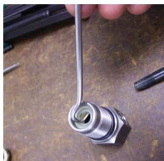
34. Pull cup seal (Item 15) out of wrist pin anchor (Item 13a).
