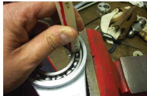
60. Drive ball bearing (Item 7) out of crank rod (Item 4).
