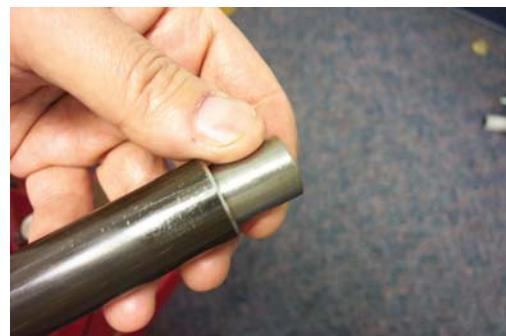
48. Remove lower plunger and bushing assembly (Item 19) from reciprocating tube (Item 20). (Reassembly recommendations: replace O-ring seal (Item 26.) Remove lower cup (Item 21) from reciprocating tube (Item 20). Remove pump bushing (Item 19a) from pump plunger (Item 19).
