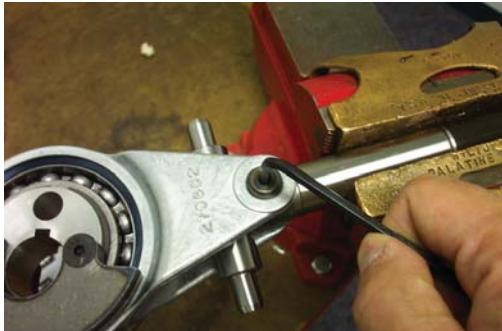
22. Remove wrist pin bushing screws (Item 11). (Reassembly torque: 100-110 in. lbs. (11.3 - 12.4 Nm).) Reassembly recommendations: use Loctite 242 or equivalent on screw threads.
