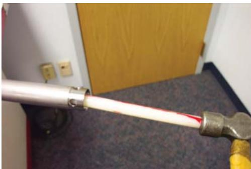
17. Push pump element (items 1 through 27) out of housing tube with plastic rod and hammer. (Reassembly recommendation: replace pump element in housing tube with housing tube slightly loose, then torque housing tube (Item 56a) to pump housing (Item 73) to 20-25 Ft. Lbs. (27.1 - 33.9 Nm).)
