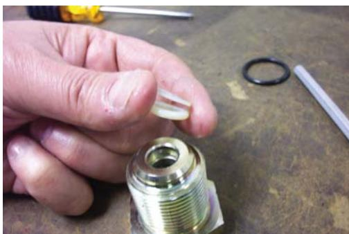
62. Remove O-ring seal (Item 34) and backup washer (Item 35) from outlet nut (Item 32). Note the position of the backup washer in photo.
