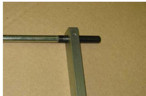
49. To remove lower plunger, use special tool provided in Tool Kit 276275.
