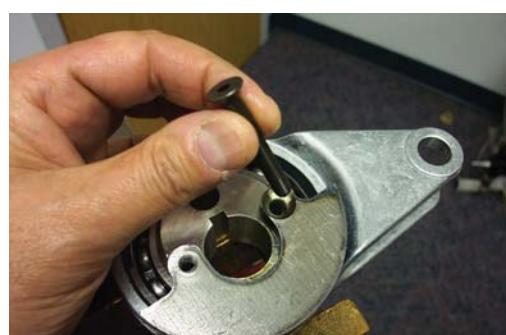
55. Remove flat head screws (Items 1). (Reassembly recom-mendation: use loctite 242 on screw threads).
