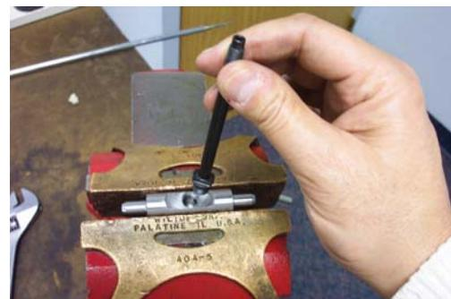
38. Remove plunger tube (Item 10). (Reassembly recommendations; replace o-ring (item 9). use Loctite 242 or equivalent on plunger tube threads.)
