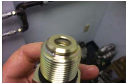
63. Reassembly recommendations: To install the O-ring (Item 34) and backupwasher (Item35) most easily, install the backup washer first.
