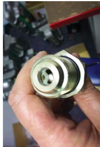
64. And then feed the O-ring (Item 34) under the backup washer, pushing up the final bulge of the O-ring with a blunt rod.
