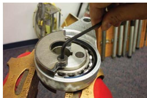
54. Loosen flat head screw (Item 1). (Reassembly torque: 100-110 in. lbs. (11.3 - 12.4 Nm).)
