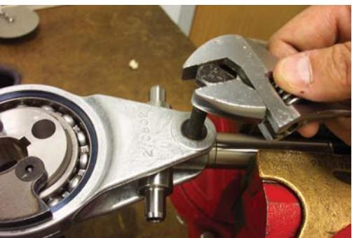
24. Press out wrist pin bushing (Item 12) with 5/16-24 bolt, needed since pivot bushings often stick in wrist pin anchor (Item 13a).
