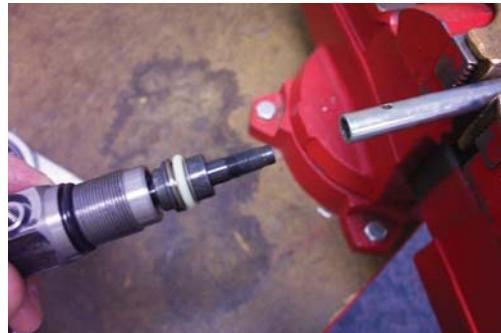
31. Remove plunger tube (Item 10) and associated parts. (Reassembly recommendations: replace O-ring (Item 10c) on bushing (Item 10a). Use Loctite 242 or equivalent on plunger tube threads.)
