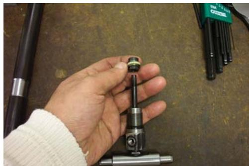
32. View of bushing assembly (Items 10 through 10d) removed.
