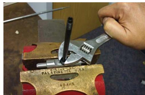
37. Loosen plunger tube (Item 10) from outlet pin (Item 8). (reassembly torque: 100-110 in.-lbs. (11.2 - 12.4 Nm).)
