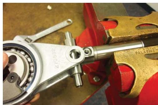
26. Remove crankrod and eccentric assembly (Items 1-7).
