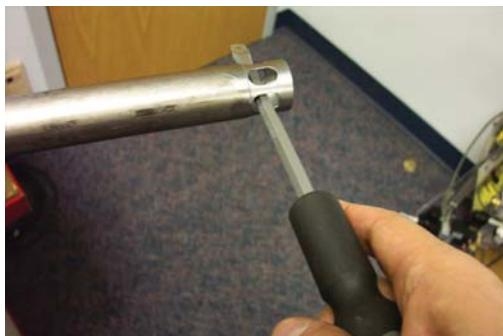
18. Remove housing tube (Item 56a). (Reassembly Torque: 20 to 25 Ft. Lbs.(27.1 - 33.9 Nm).)
