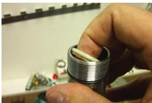
21. Remove oil seal O-ring (Item 53) and backup washer (Item 59). (Reassembly recommendation: replace O-ring seal and backup washer, backup washer must be placed in tube first, then the O-ring.)
