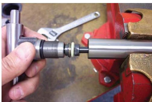
29. View of plunger tube and plunger tube bushing assembly (Items 10, 10a, 10b, 10c and 10d).
