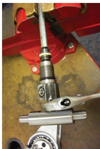
30. Loosen plunger tube (Item 10). (Reassembly torque: 100-110 in. lbs. (11.3 - 12.4 Nm)).
