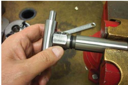
28. Remove wrist pin anchor (Item 13a). (Reassembly recommendations: replace O-ring seal (Item 13b), be sure threads on wrist pin anchor (Item 13a) are clean and free of all oil or other fluids.)
