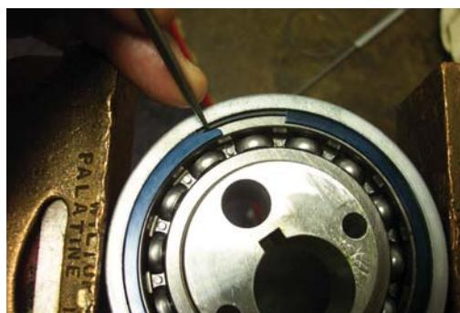
57. Remove inner and outer retaining ring (Item 5 and Item 3) from both sides.
