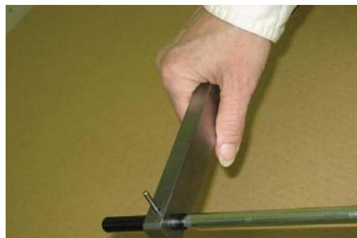
51. Remove plunger (Item 19). (Reassembly torque: 100-110 in. lbs. (11.3 - 12.3 Nm)) (Reassembly recommendations: use Loctite 242 or equivalent on plunger threads)
