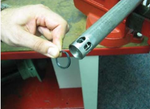
15. Remove spiral retaining ring (item 59) from housing tube.
