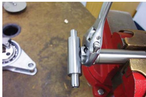
27. Loosen wrist pin anchor (Item 13a). (Reassembly torque: 20 - 25 Ft. Lbs. (27.1 - 33.9 Nm).)
