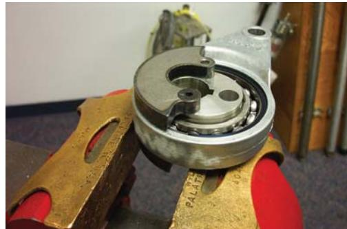
53. Clamp crank rod/eccentric assembly (Items 1-7) in vise.
