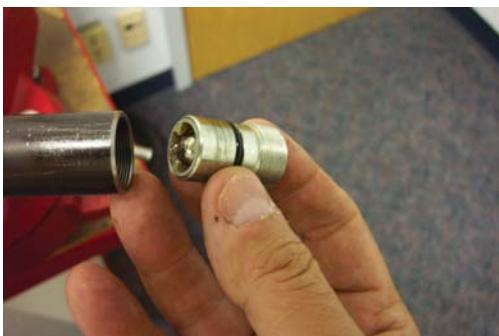
46. Check seat housing assembly (Item 27) and associated parts removed. (Reassembly recommendations: replace O-ring seal (Item 26). Apply Loctite 242 or equivalent to check seat housing threads.)
