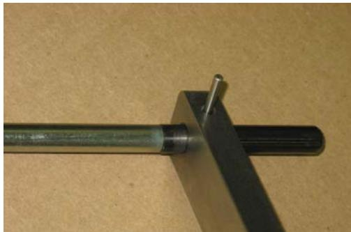
50. With the tool in place, insert the 9/64" drill bit shank through the tool and into the plunger outlet hole.
