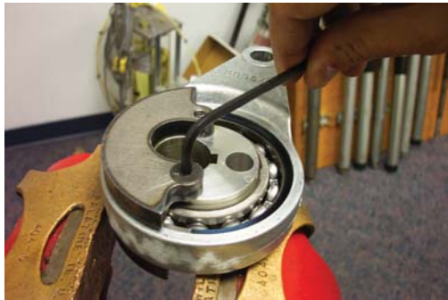
63. Loosen flat head screw (Item 1). (Reassembly torque: 100-110 in. lbs.)
