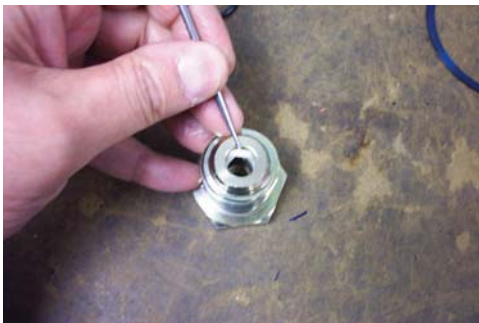
70. Remove O-Ring seal (Item 33) from outlet nut (Item 32).
