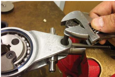
33. Press out wrist pin bushing (Item 12) with 5/16-24 bolt (from 276275 kit), needed since pivot bushings often stick in wrist pin anchor (Item 13a).
