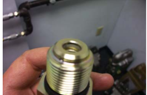
72. Reassembly recommendations: To install the O-ring (Item 34) and backupwasher (Item35) most easily, install the backup washer first.
