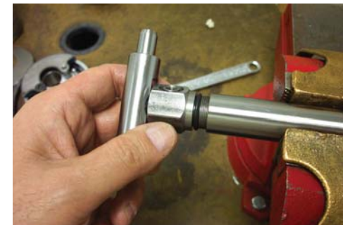
37. Remove wrist pin anchor (Item 13a). (Reassembly recommendations: replace O-ring seal (Item 13b), be sure threads on wrist pin anchor (Item 13a) are clean and free of all oil or other fluids.)
