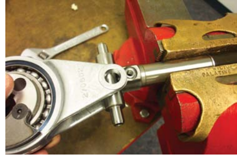
35. Remove crankrod and eccentric assembly (Items 1-7).
