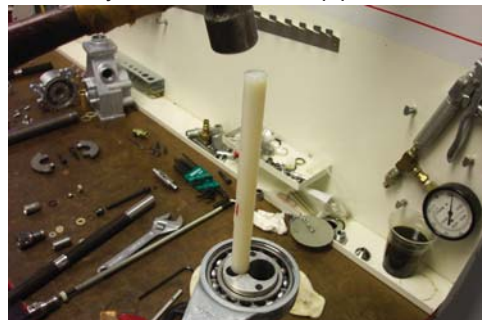
68. Drive crank eccentric (Item 6) out of ball bearing (Item 7).
