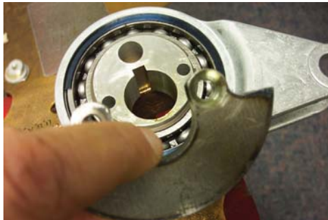
64. Remove flat head screws (Items 1). (Reassembly recommendation: use loctite 242 on screw threads).
