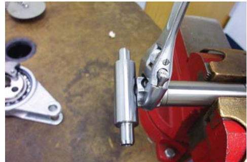
36. Loosen wrist pin anchor (Item 13a). (Reassembly torque: 20 - 25 Ft. Lbs. (27.1 - 33.9 Nm).)
