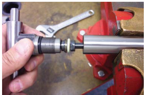
38. View of plunger tube and plunger tube bushing assembly (Items 10, 10a, 10b, 10c and 10d).
