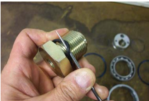
70. Remove O-Ring seal (Item 33) from outlet nut (Item 32).
