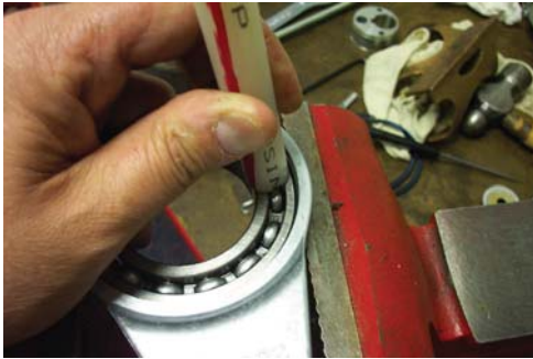
69. Drive ball bearing (Item 7) out of crank rod (Item 4).
