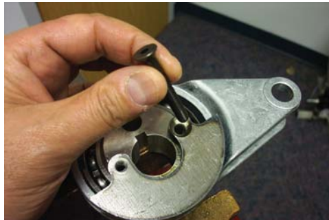
64. Remove flat head screws (Items 1). (Reassembly recommendation: use loctite 242 on screw threads).
