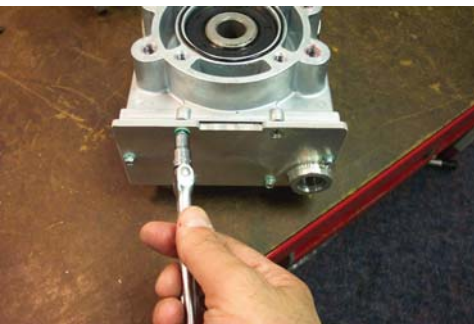
10. Remove housing cover screws (Item 28). (reassembly recommendations: replace screw gaskets(item 29))
