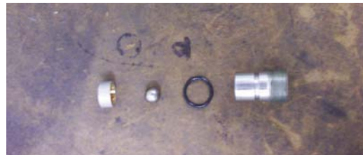
56. Remove ball cage (Item 24), check ball (Item 25) and O-ring seal (Item 26) from check seat housing (Item 27).
