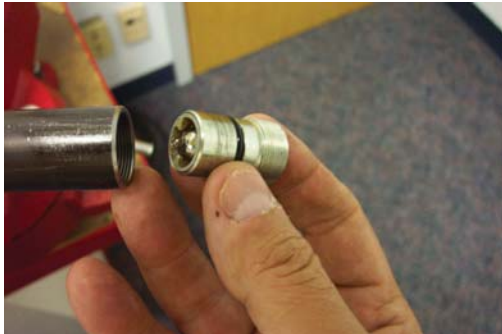
55. Check seat housing assembly (Item 27) and associated parts removed. (Reassembly recommendations: replace O-ring seal (Item 26). Apply Loctite 242 or equivalent to check seat housing threads.)
