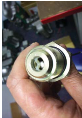
73. And then feed the O-ring (Item 34) under the backup washer, pushing up the final bulge of the O-ring with a blunt rod.
