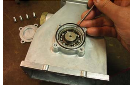
14. Remove bearing cover O-ring (Item 63). (Reassembly recommendations: replace bearing cover O-ring.)
