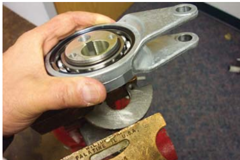
65. With both flat head screws removed, remove counterbalance weights (Item 2).
