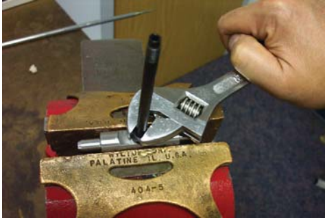
46. Loosen plunger tube (Item 10) from outlet pin (Item 8). (re-assembly torque: 100-110 in.-lbs. (11.3 - 12.4 Nm).)
