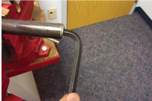
54. Loosen check seal housing (Item 27) with 3/8 Allen wrench. (Reassembly torque: 20-25 ft. lbs.(27.1 - 33.9 Nm).)
