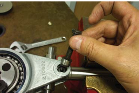
34. Remove wrist pin bushing (Item 12).
