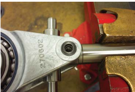
32. View of wrist pin bushing (Item 12).
