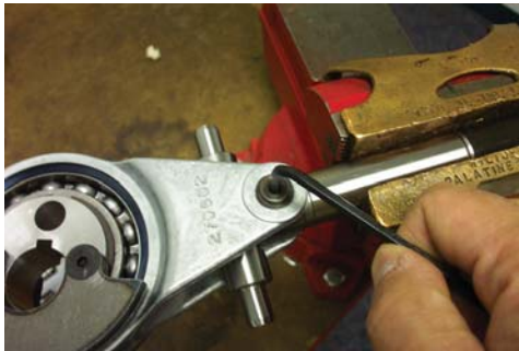
31. Remove wrist pin bushing screws (Item 11). (Reassembly torque: 100-110 in. lbs. (11.3 - 12.4 Nm).) Reassembly recommendations: use Loctite 242 or equivalent on screw threads).
