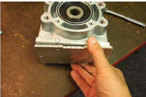
11. Remove housing cover (item 30) and Gasket (Item 31). (Reassembly recommendation: replace gasket)
