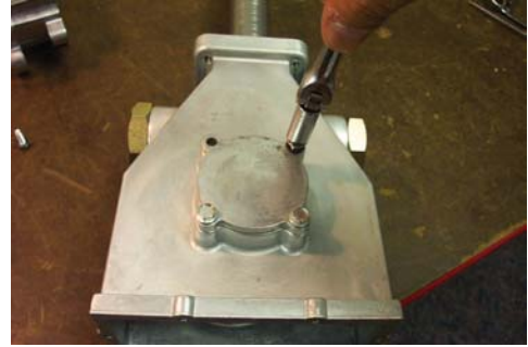
12. Remove bearing cover screws (Item 66) with lockwashers (Item 65). (Reassembly torque: 32-38 in. lbs. (3.6 - 4.3 Nm).)
