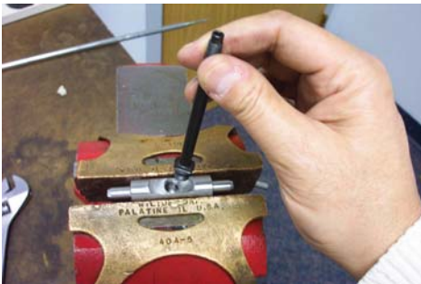
47. Remove plunger tube (Item 10). (Ressembly recommendations; replace o-ring (item 9). use Loctite 242 or equivalent on plunger tube threads.)
