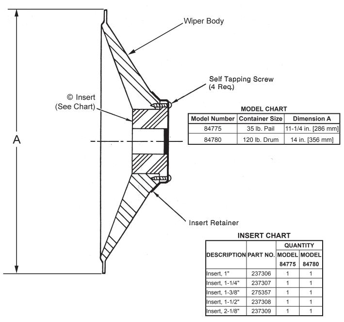
NOTE: When using the follower with an 81384 pump, it may be dfficult to remove the follower from an empty pail of grease unless the seal is broken between the follower lip and the container. This can be done by removing the lid and pump and rocking to loosen seal, or by inserting a blunt object between the follower lip and container.
