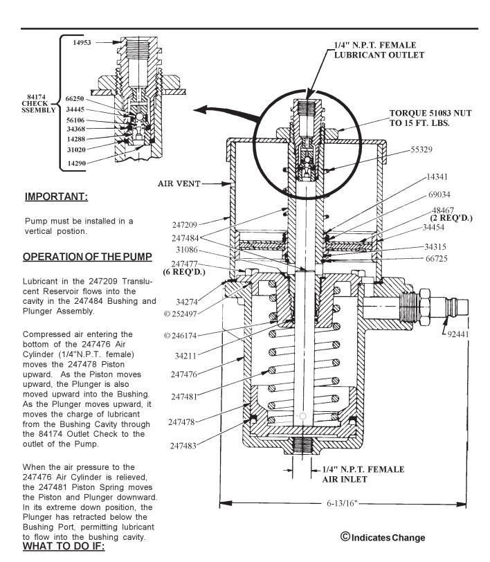
Pump loses prime. - Check lubricant supply.
