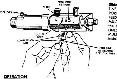
Slide COMPRESSION NUT over FEED LINE. Insert FEED LINE into OUTLET PORT of MULTI-LUBER BODY. Hold FEED LINE securely against STOP in MULTI-LUBER BODY while hightening the COMPRESSION NUT. All FEED LINES must be connected to the MULTI-LUBER before RESERVOIR is installed.
