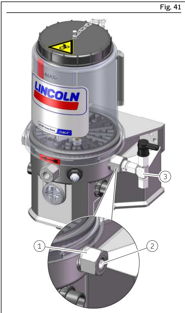
Replacing pump element and pressure limiting valve
