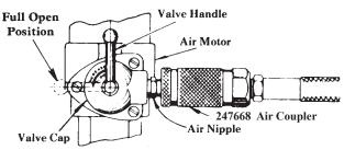
Uncouple 247668 Air Coupler from air nipple. Fill air coupler with No. 10 S.A.E. Motor Oil. Quickly recouple to air nipple. Normal operation of pump will carry the oil to all parts of the air motor which require lubrication.
