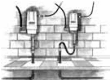
Standpipe and wall mount assembly to remote bulk tanks
